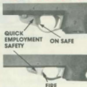
It disconnects the trigger. It can be moved "off safe" very quickly with the trigger finger. It provides safety even when instant readiness is needed. You can have it "on safe" while the carry safety is "on safe" so it will already be "on" when you disengage the carry safety.
