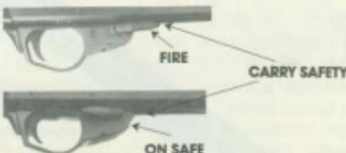
The carry safety should only be engaged when the **SAS 12** is cocked. With bolt closed and hammer **UNCOCKED**, engaging the carry safety prevents opening the bolt and cocking the gun.
